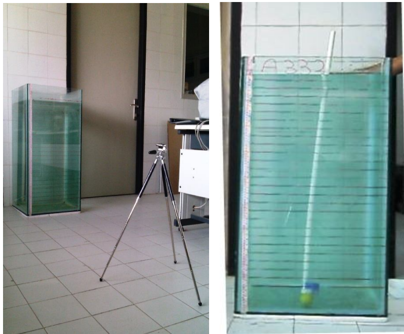
Figure 1. Water column for determination of hydrodynamic properties. An apple on the bottom of the water column, prepared to be released.
