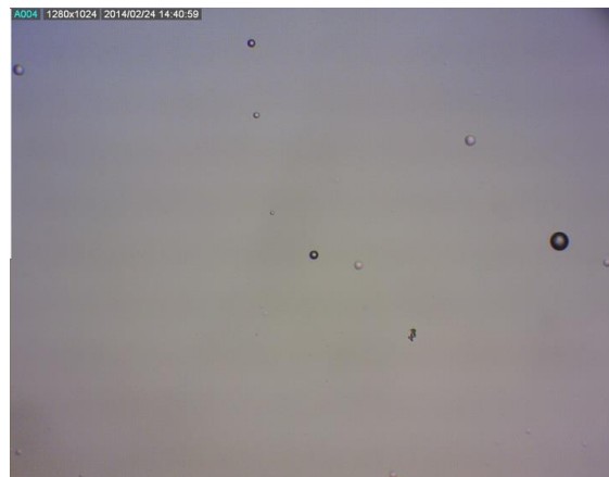
Fig. 2. Neutron microscopic traces on the surface of a CR-39 film
