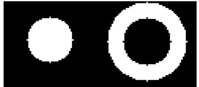
Fig. 1: ICRU Sphere phantom (radius 15 cm) and a radioactive source (internal radius 15 cm and external radius 25 cm).
