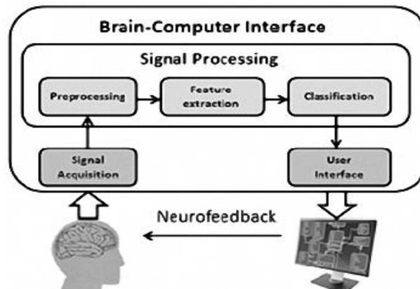
Fig. 1. BCI block diagram (Kolodziei et al., 2012).
